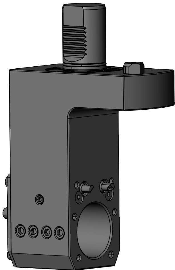
90 DEGREE VDI40 STATIC TOOL OUTPUT: 2" BORING BAR COOLANT: EXTERNAL & INTERNAL **BACK PLATE REMOVABLE**
